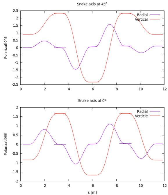
Figure 3. The closed orbits inside a snake: (top)  $45^\circ$  snake axis angle; (bottom)  $0^\circ$  snake axis angle.
