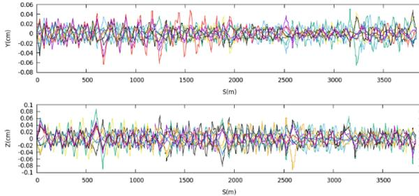
Figure 5: Trajectory: radial (top) and vertical (bottom) closed orbit excursions around RHIC for 10 different random seeds.
