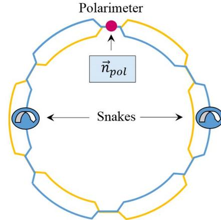
Figure 1: RHIC ring with two helical snakes.
