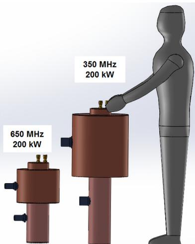
Figure 6: Solid models of 350 MHz and 600 MHz RF sources using the water-cooled, multiple beam triode of Fig. 5.
