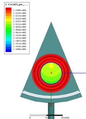
Figure 8: Electric field variation across multiple beam triode grid.
