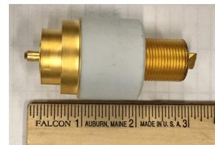
Figure 2. YU-176 triode produced by Communications & Power Industries, LLC.
