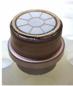
Figure 3: Grid-cathode assembly for YU-176 triode.
