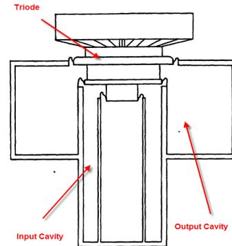
Figure 1: Schematic configuration of triode-base RF source.
