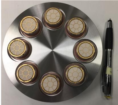
Figure 4: Eight grid-cathode array for multiple beam triode.
