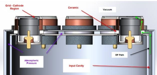
Figure 7: Grid-cathode region of multiple beam triode showing path of RF drive signal.
