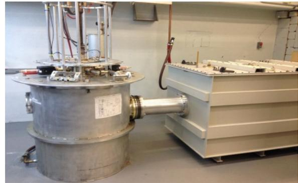
Figure 1: 500 kV, 218 A electron gun tank (at left) connected to the 500 kV, 250 A Marx modulator (at right) in the Beam Physics Lab at Yale University.
