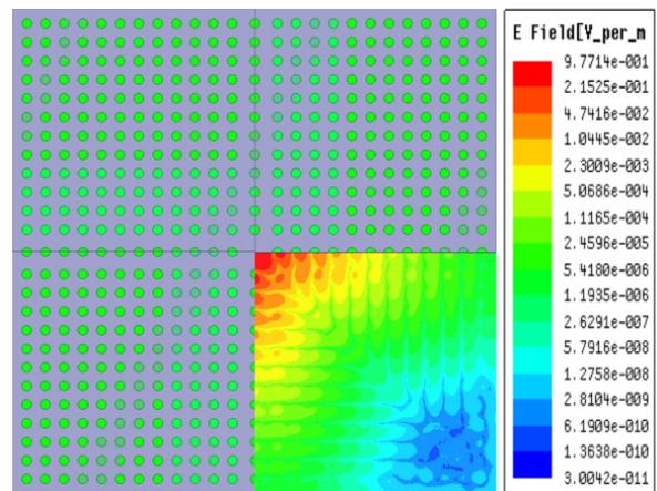
Figure 11: Structure and E-field distribution (logarithmic scale) of operating eigen mode in resonator consisted of 12 layers of rods.
