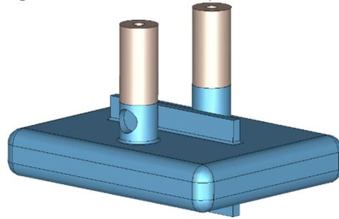
Figure 1: X-band copper resonator for Meissner qubit.
