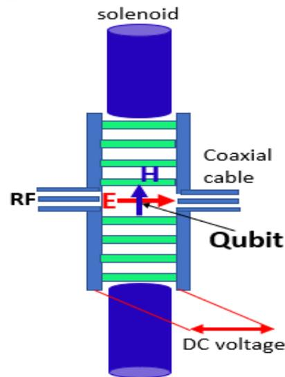
Figure 6: Sketch of sapphire resonator with SRF walls and DC electric or magnetic bias.
