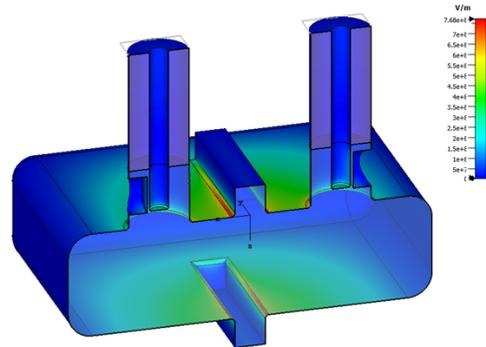
Figure 2: Surface electric field of the eigen mode.
