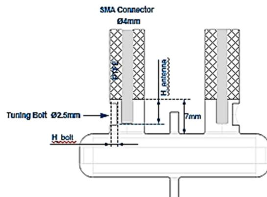
Figure 3: Drawing of X-band copper cavity.
