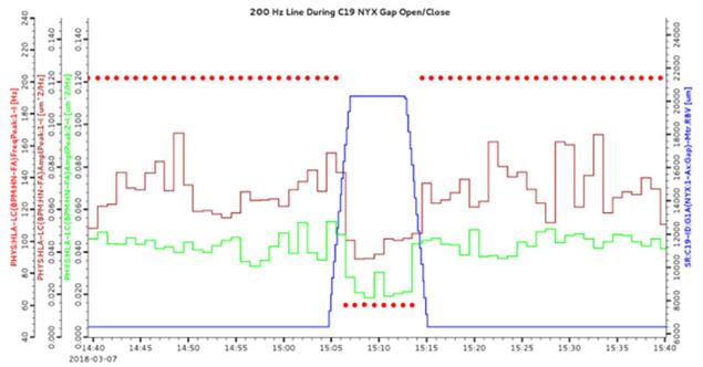
Figure 6: The frequency (red circles) and amplitude of the highest (brown) and the 2nd highest (green) spectral peaks for hor. non-dispersive BPMs. The 19-ID (NYX) undulator gap (blue) is fully opened and then fully closed.
