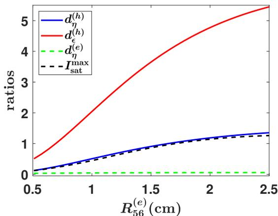
Figure 4: Diffusion and saturation ratios versus the common e-chicane strength. As far as the former is concerned, we define  $d_\eta^{(h,e)} = (T/\sigma_h^2) \langle D_\eta^{(h,e)} \rangle_z / \langle 1/N_c^n \rangle_z$  etc.
