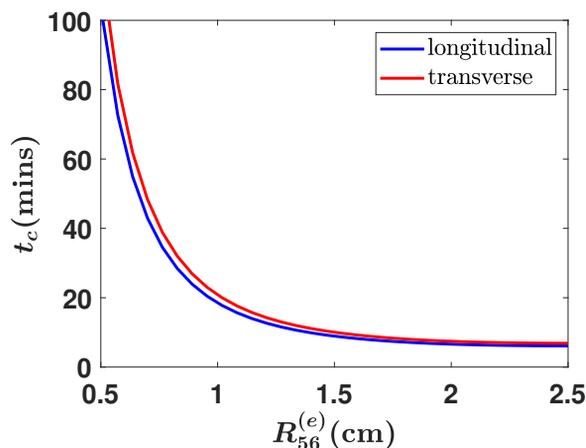
Figure 3: Bunch-averaged cooling times vs the common value of the electron chicane strengths.
