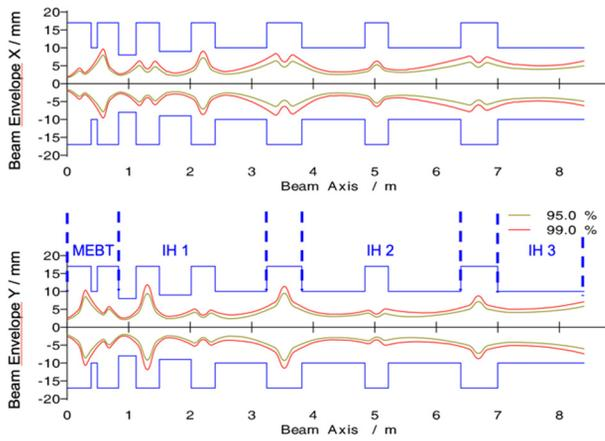
Figure 3: Transverse beam envelopes RFQ exit to IH3 exit.
