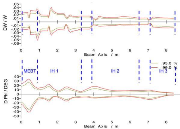
Figure 4: Longitudinal beam envelopes RFQ exit to IH3 exit.
