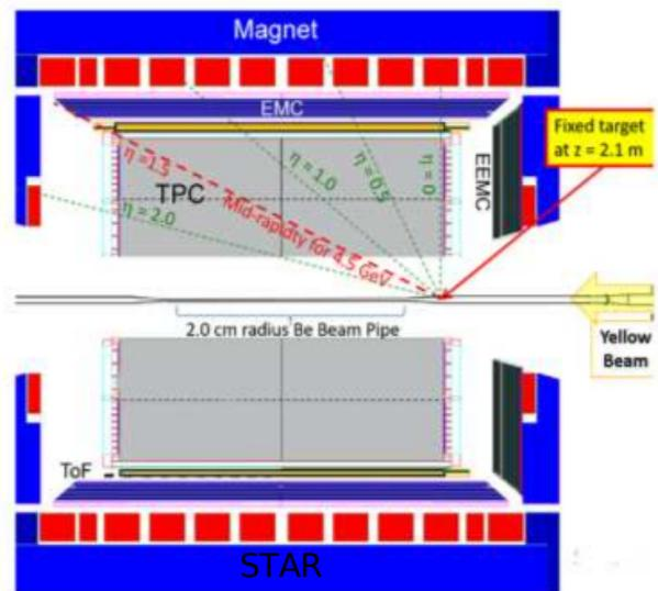
Figure 1: The fixed target layout with respect to the RHIC ring and STAR detector.
