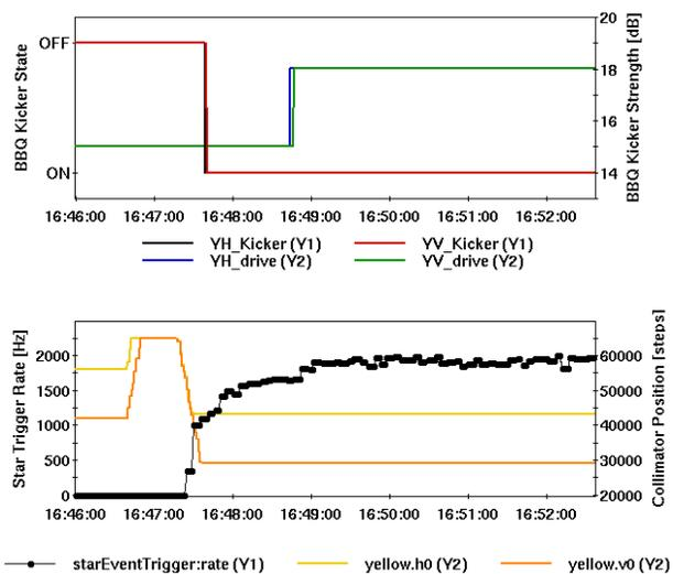
Figure 5: The trigger rate reaches 2000Hz with help of the BBQ kickers shortly after the collimators were pulled out.
