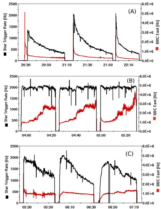
Figure 7: The BBC East rates were the limiting factor in keeping the STAR trigger rate leveled. (A) The trigger rate with the BBQ kickers off. (B) The trigger rate is being leveled at 2000Hz using BBQ without considering the background level. (C) The emphasis is put on keeping the background within limits and thus the 2000Hz trigger rate can not be maintained.
