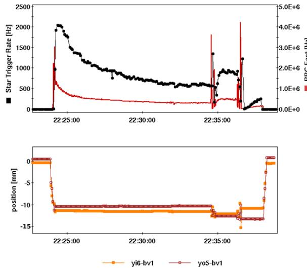
Figure 3: An attempt to control the trigger rates by using the orbit control. Vertical position of the beam is described here by two BPMs, yi6-bv1 and yo5-bv1, which are approximately  $\pm 25$  m from STAR. Even small changes in orbit lead to spikes in the trigger rate and detector signals (BBC East is one of the STAR sub-detectors).
