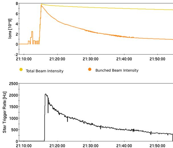
Figure 2: The STAR trigger rate is strongly correlated with the bunched beam intensity.
