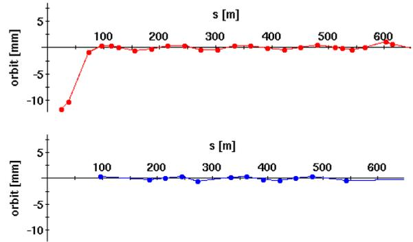
Figure 4: An example of the vertical BPM signal. Horizontal axis is a location around the RHIC ring with  $s(\text{STAR}) = 0$  m. Yellow beam travels right-to-left. Top - beginning of the store; Bottom - end of the store (approximately 30 minutes later), some BPMs stop reporting as the beam de-bunches.
