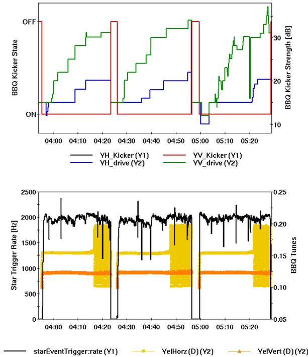
Figure 6: The trigger rate maintained by use of the BBQ kickers. Both horizontal and vertical planes were used and the kicker strength was varied. Allowing almost continuous betatron tune measurement.
