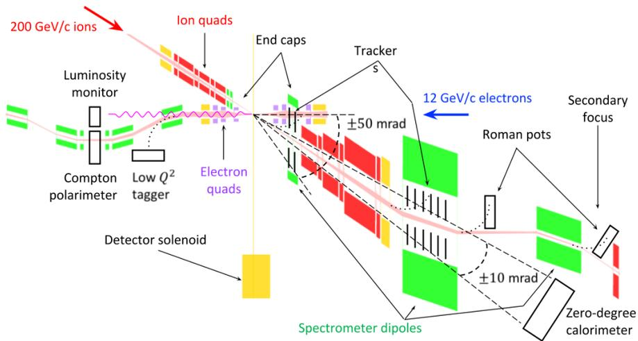
Figure 1: JLEIC detector region elements layout.
