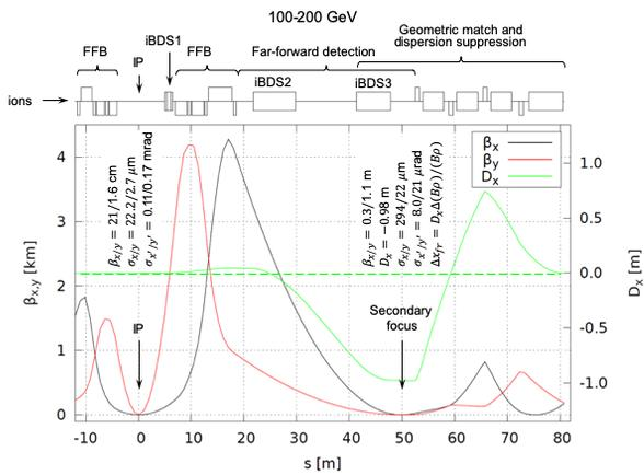
Figure 2: Beam optics of the ion detector region. Also shown are the positions of the IP and secondary focus, and the beam parameters at those locations.
