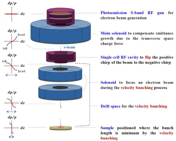
Figure 4: The design concept of bunch compression with a single-cell RF cavity.
