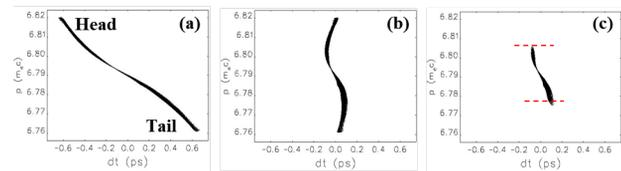
Figure 2: Longitudinal phase spaces; (a)  $\sigma_z = 317$  fs (rms) at the entrance of the alpha-magnet; (b)  $\sigma_z = 56$  fs (rms) at the exit of the alpha-magnet without energy slits; (c)  $\sigma_z = 47$  fs (rms) at the exit of the alpha-magnet with energy slits.
