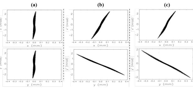
Figure 3: Transverse phase spaces; (a)  $\epsilon_{nx} = 50$  nm,  $\epsilon_{ny} = 50$  nm at the entrance of the alpha-magnet; (b)  $\epsilon_{nx} = 50$  nm,  $\epsilon_{ny} = 50$  nm at the exit of the alpha-magnet without energy slits; (c)  $\epsilon_{nx} = 55$  nm,  $\epsilon_{ny} = 59$  nm at the exit of the alpha-magnet with energy slits.
