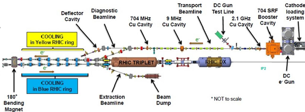
Figure 2: Layout of the LEReC accelerator.
