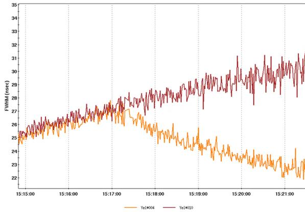
Figure 3: Time evolution of ion bunch length (full-width half maximum, nsec). Uncooled ion bunch – top brown curve (Yel#004). Cooled bunch – low yellow curve (Yel#10). Electron and ion velocities are matched at 15:17.
