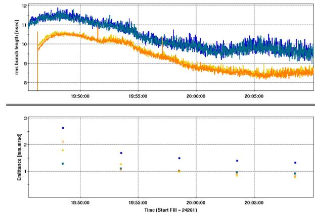
Figure 4: 6-D cooling of a 111x111 bunch RHIC store at 3.85 GeV (1.6 MeV electrons, 15mA 9 MHz CW current). Top plot - reduction of bunch length. Bottom plot - reduction of transverse beam emittances (two rings, two planes).
