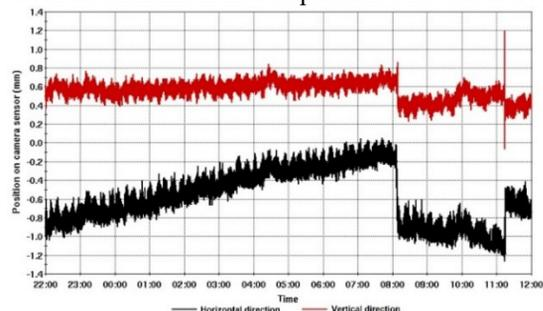
Figure 1: Example data of CoM laser position (horizontal position in black, vertical position in red) during operations without active pointing stabilization, showing fast fluctuations, slow drifting, and user corrections.
