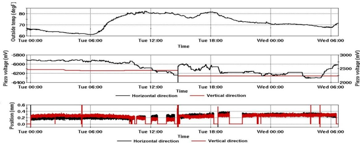
Figure 2: Example of pulsed operations during the 2019 Run with slow stabilization active. Top plot - outside temperature. Middle plot - piezo commands sent to steering mirrors (includes user commands). Bottom plot - beam position on camera sensor, which is logged as zero when there is no beam (e.g. closed shutter).
