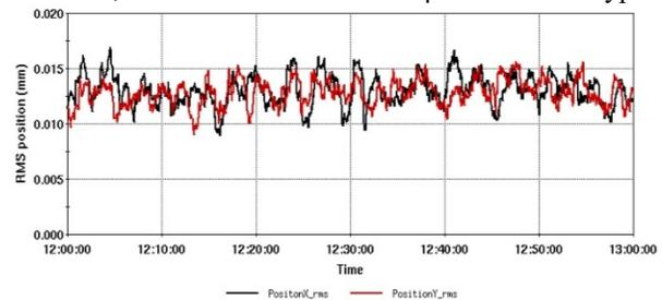
Figure 3: RMS CoM position with fast stabilization active.
