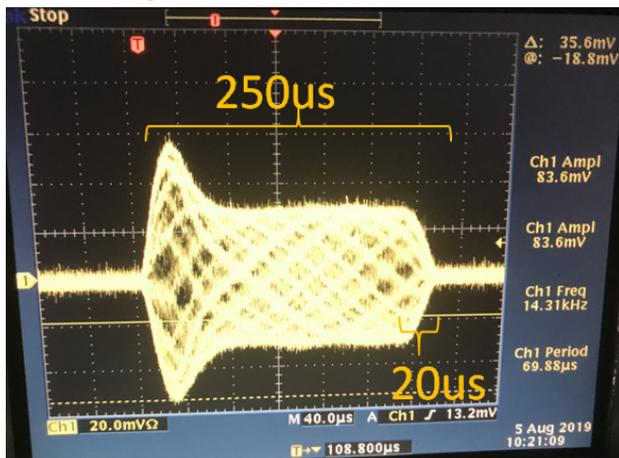
Figure 6:  $250\mu\text{s}$  macro pulse signal measured at the hot deck.
