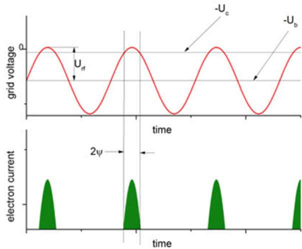
Figure 4: Voltages applied to the grid (top). When this exceeds the cut off,  $U_c$ , emission occurs (bottom).
