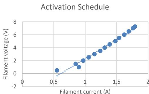
Figure 7: Plot of cathode activation.
