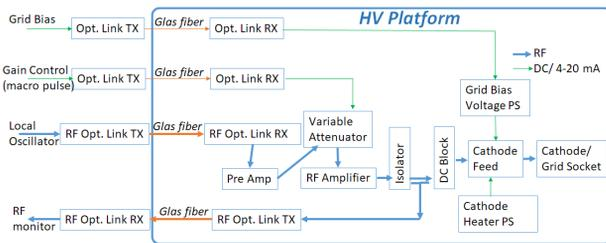
Figure 3: RF Cathode and grid drive design.
