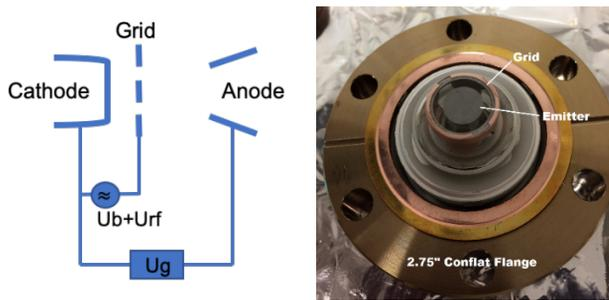
Figure 2: (left) Gun electrical diagram,  $U_b$ : bias voltage,  $U_{rf}$ : RF voltage,  $U_g$ : Gun voltage. (right) Gridded cathode (CPI Y-845).
