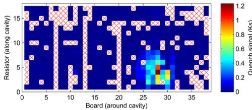
Figure 3: A quench map of a Nb<sub>3</sub>Sn cavity showing localized heating into the bottom right sector. This demonstrates to localized area of the quench. Note: red x's show thermometers that failed during the test.
