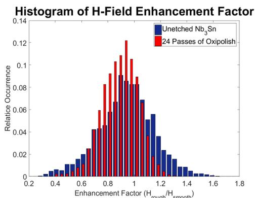
Figure 6: Histogram of magnetic field enhancement of  $Nb_3Sn$  and oxypolished  $Nb_3Sn$  [14]. The y-axis shown the relative fraction of surface at a field enhancement value.
