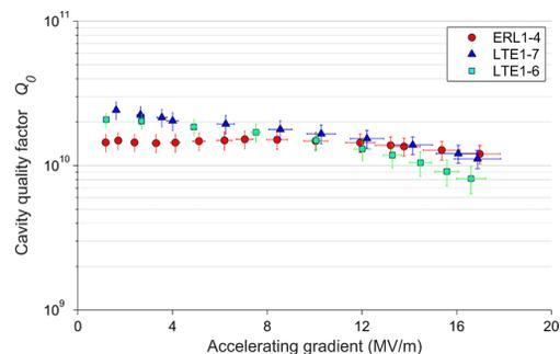
Figure 2: Q vs. E at 4.2 K of several 1.3 GHz TESLA elliptical cavities made at Cornell University.
