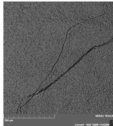
Figure 5: SEM scan of a quench site cut out from a cavity. The black lines are likely Nb substrate grain boundaries.
