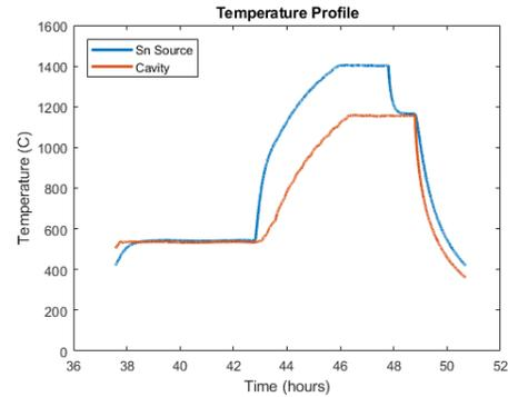
Figure 1: Temperature profile from the coating of a Nb<sub>3</sub>Sn cavity. Both the temperature of the cavity and the Sn source are shown.
