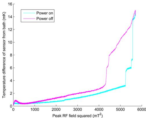
Figure 4: Measuring the temperature rise at the quench site (outside surface) with respect to time as the RF field rises (cyan) and then falls (magenta) in the cavity. The cavity does not quench during the cycle. Temperature jumps are present at higher RF field levels (near quench).
