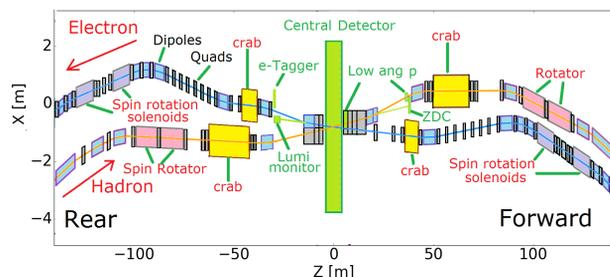
Figure 1: Schematic view of the eRHIC interaction region (top view). Note the different scales on the two axes.
