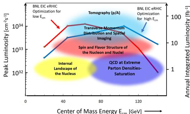
Figure 2: Luminosity vs. center-of-mass energy for two different optimizations of the interaction region and beam parameters. The blue curve, which shows an optimization at 105 GeV CM energy, is based on 1160 bunches and 25 mrad crossing angle, while the red curve, optimized at 63 GeV, is based on 2320 bunches and 50 mrad crossing angle.
