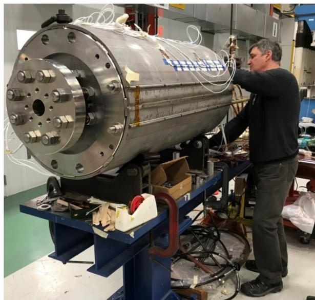
Figure 1: 15 T dipole demonstrator MDPCT1.
