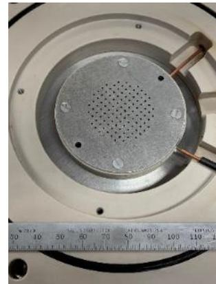
Figure 1: Extraction column with total of 120 beamlets (each of which is 0.5 mm in diameter, and 3 mm center-to-center spacing).
