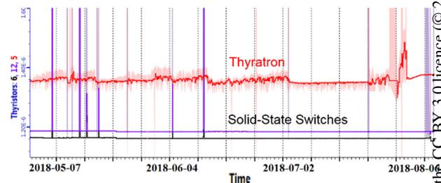
Figure 4: Kickers 6 and 12 thyristor and kicker 5 thyatron jitter over 100 days. Thyristors ±2 ns, thyatron at ±50 ns by end of life.
