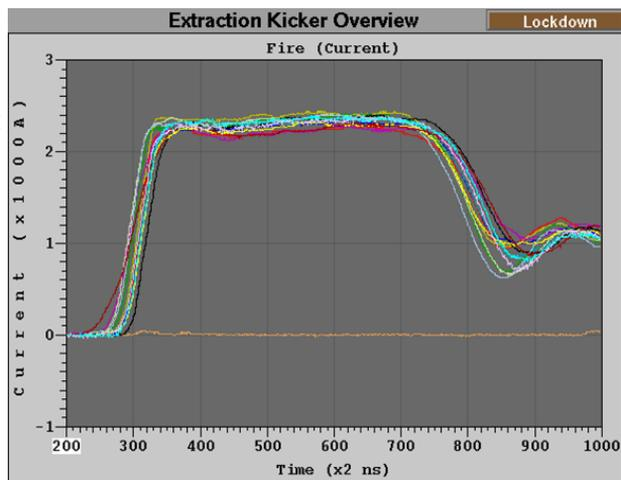
Figure 6: Magnet currents for 14 kickers (1 is spare and out of time) matching rise times. 1000 A/division, 100 ns/division.
