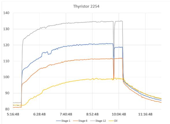
Figure 2: Temperature testing of thyristor, stages 1, 6, and 12 shown. Stages 1 and 6 are below 120°F while stage 12 is above 135°F. Differences in temperature are attributed to cooling flow differences between each stage.
