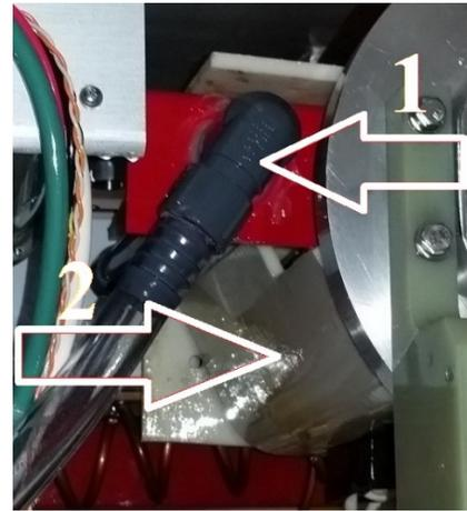
Figure 3: Thyristor baffling and manifold. Manifold is indicated by arrow at location 1 and baffling by arrow at location 2.
