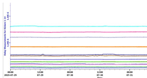
Figure 5: All 14 kickers' jitter/drift after conversion over 2 days.
