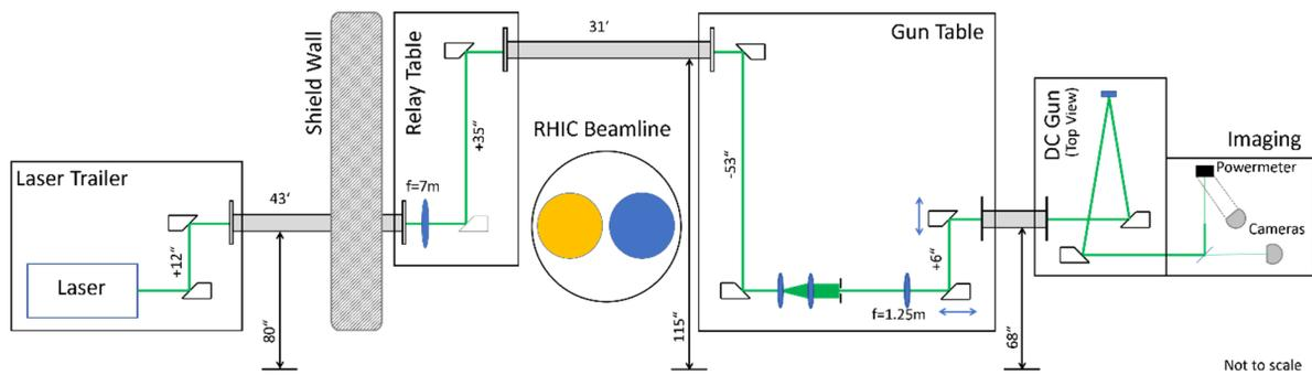
Figure 1: Schematic of the LEReC Laser Transport System.
