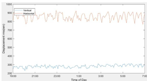
Figure 2: Overnight vibration measurement on the optical table surface in the trailer before the mounting of the table on the steel block below ground.
