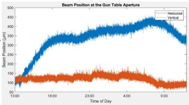
Figure 6: Measurement of an alignment beam position at the gun table over the course of a day relative to the centre of the camera sensor.
