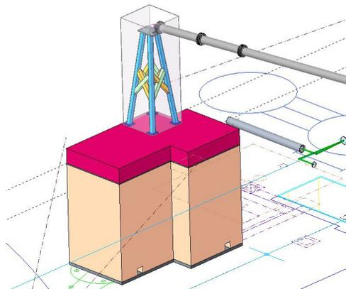
Figure 3: Rendering of the gun table, including incoming transport pipe and A-Frame to lower the incoming beam onto the table.
