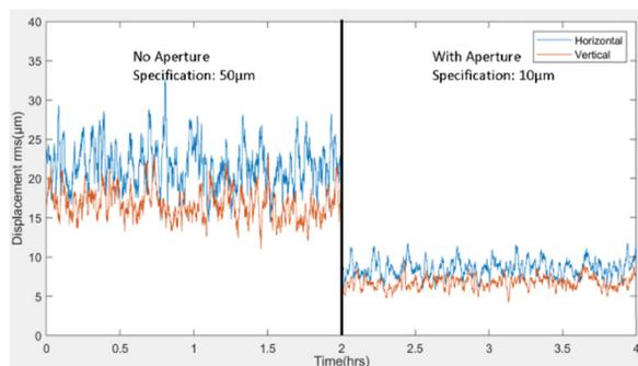
Figure 5: Measurement of the rms position of an alignment laser transported to the gun table at the location of the aperture that is imaged to the photocathode.
