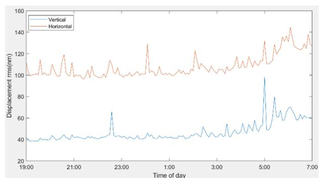
Figure 4: Overnight vibration measurements of the optical table surface after mounting of the table on steel blocks below ground. Anomalies in the measurements starting around 5:00 are due to work in the vicinity of the trailer.
