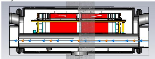
Figure 5: Cut view of PAR septum. The stored beam is indicated by arrows. Injected (from right) and extracted (to the left) are through the top beam pipes.
