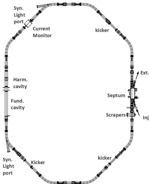
Figure 1: Layout of the PAR vacuum chamber.
