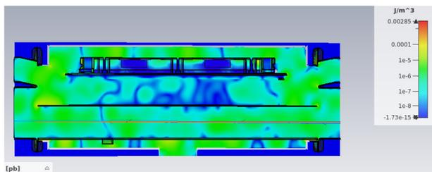
Figure 6: Electric field energy after 31 ns of beam entry. The field level is very weak.
