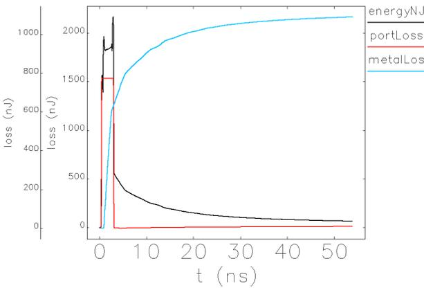
Figure 4: Stored energy and integrated metal and port losses vs time of the kicker chamber.
