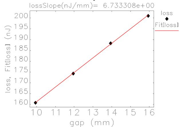
Figure 8: Loss factor gap scan result.
