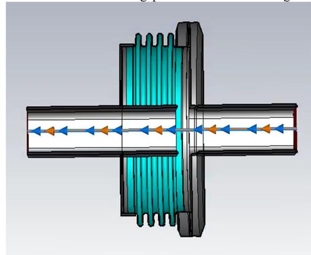
Figure 7: PAR chamber bellow flange with a 6 mm gap between the liner (left) and a right chamber.
