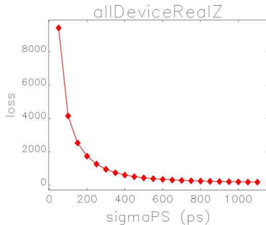
Figure 2: Energy loss of a 1 nC beam vs bunch length. At 1 ns bunch length the loss is 185 eV.
