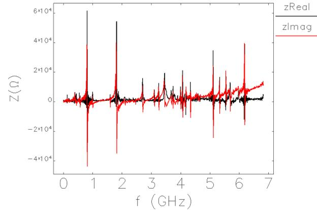
Figure 3: Real and imaginary total impedance of the PAR.
