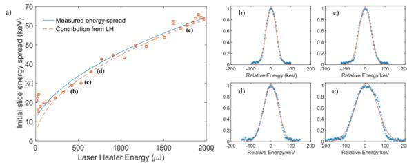
Figure 2: (a) Slice energy spread of the e-beam after the laser heater as a function of LG01 beam energy; and (b-e) four examples energy distributions in (a) with 25.1 (b), 30.3 (c), 36.8 (d), and 55.7 (e) keV energy spread and their corresponding Gaussian fits.
