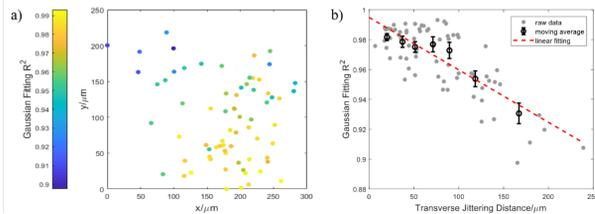
Figure 5: Influence of transverse laser jitter for LG01 mode laser heater. (a) Positions of laser center on the camera of different shots with Gaussian fitting  $R^2$  of their corresponding induced energy distributions. (b) Correlation between the Gaussian fitting  $R^2$  of the energy distribution and radial distance laser jittering away from the optimal position.
