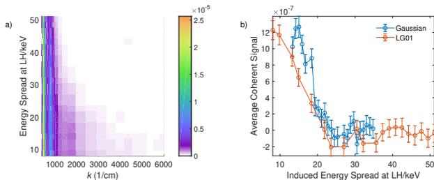
Figure 3: a) 2D-MIR spectrograph as a function of induced energy spread by LG01 transverse mode LH and b) integrated MIR spectral intensity for  $k \in (3000, 5000) \text{ cm}^{-1}$  as a function of induced energy spread by both the LG01 and Gaussian mode LHs.
