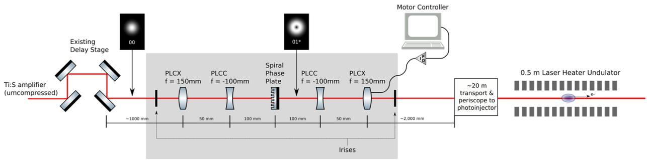
Figure 1: Simplified optical mode-conversion and control systems schematic, and transport to the laser heater undulator at the LCLS photoinjector
