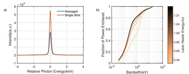
Figure 4: a) Averaged (red) and single shot (blue) SXRSS spectral distributions centered at 750 eV photon energy, and b) fraction of SXRSS spectral power as a function of bandwidth for varying LG01 mode energy in the LH.
